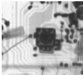
Geometric magnification with microfocus generator
