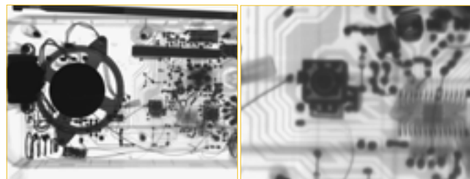
Geometric magnification with microfocus generator
